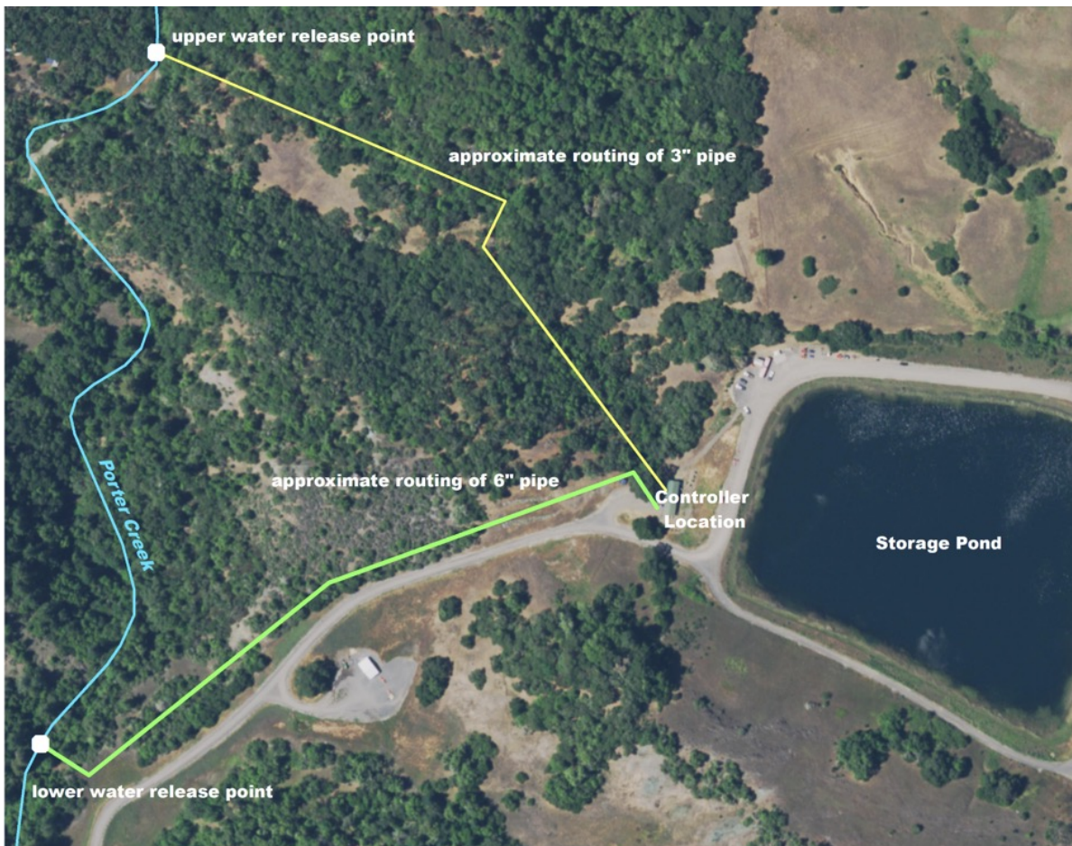
Figure 4. Schematic of approximate locations of pipe and water release points to Porter Creek from the E & J Gallo storage pond.
